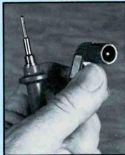
Figure 5. The design of some test probes minimizes the possibility of electric shocks. A plastic collar on the probe at left prevents fingers from sliding down the probe handle and touching the metal tip during measurements. The male banana plug (at right) is covered by plastic so no bare metal is exposed at the meter. This probe comes with Beckman meters.
