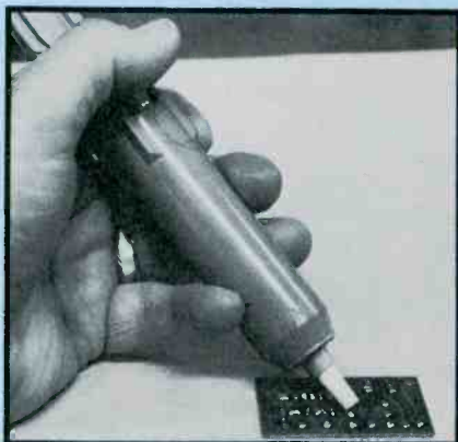
Figure 8. Spring-propelled vacuum pumps can remove solder from joints effectively, but some types might produce static electricity. This should be investigated before using any vacuum tool on FET or CMOS ICs.
