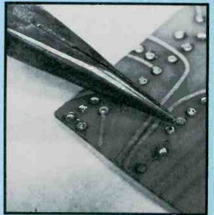
Figure 10. After braid or vacuum desolderers have removed all possible solder from a joint that has a component lead, but the lead remains stuck, use long-nose pliers to shake the lead in all four directions. When a soft pop is heard, the pin will be free and ready for removal.
