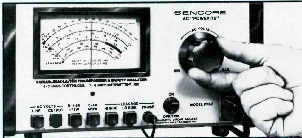
Figure 17. Sencore model PR-57 Powerite also supplies metered variable ac voltages, but in addition, measures wattage, performs leakage safety checks and provides isolated power.
