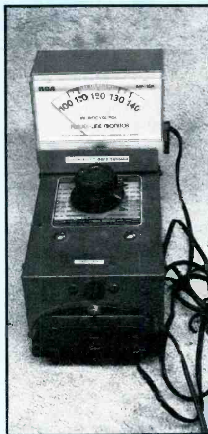
Figure 16. This old variable-transformer/ac-meter combination has provided adjustable voltage between 0V and 120V RMS for years. However, it has no isolation function, so it is dangerous to use with hot-chassis receivers.
