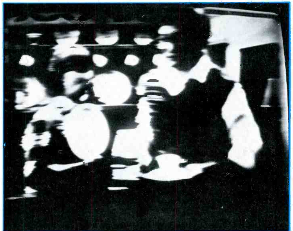
A "gassy" CRT results when the center of the cathode wears before the outside edges, causing non-linear gray-scale response.
