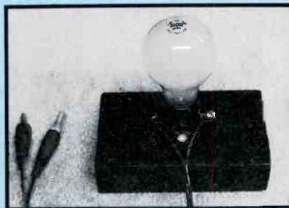
Figure 14. One method of obtaining time for locating the source of serious shorts and overloads is to limit the voltage or current. An ordinary 100W light bulb reduces both voltage and current. In addition, the bulb shows the extent of the overload by its brightness. The schematic could not be more simple, but it is recommended that you mount the bulb socket on something that is not easily tipped over. Also, insulate the alligator clips for safety.
