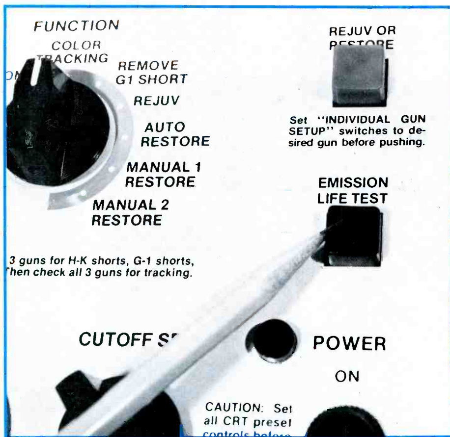
The life test on a CRT tester reduces the filament voltage to isolate temperature-sensitive cathodes, which indicate light poisoning or depleted emitting material.
