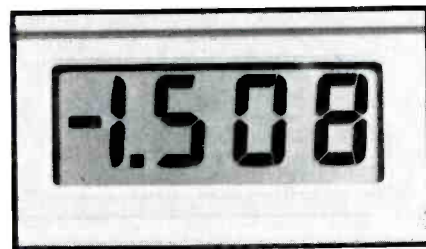
Polarity symbols appear automatically. These readings were obtained by reversing the probes on a D battery.
